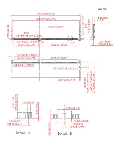
(All dimensions are in millimeters with  $\pm 0.15$ mm tolerance unless specified otherwise.)
