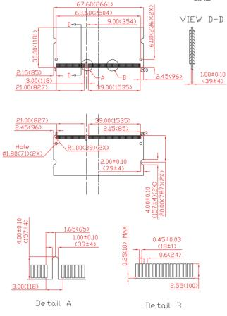
(All dimensions are in millimeters with  $\pm 0.15$ mm tolerance unless specified otherwise.)
